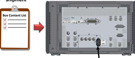
Connect the power cable to AC outlet & rear panel of the unit
